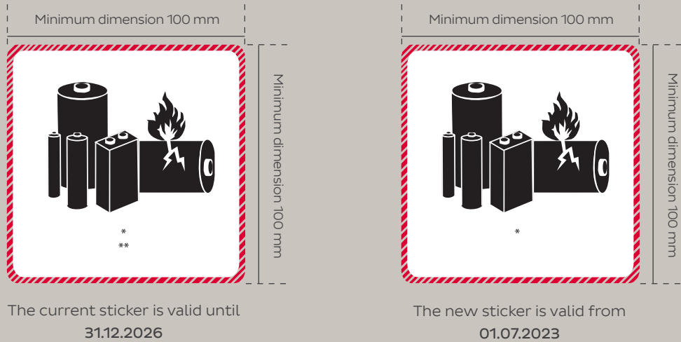
Figure according to 5.2.1.9.2 of the ADR
